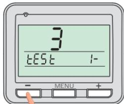
Send a signal to the receiver by pushing the **-** button.
