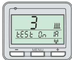
Both LEDs turn on simultaneously several times and the output relay turns on and off multiple times. "rest On / test Off" appears alternately on the display of the thermostat.
