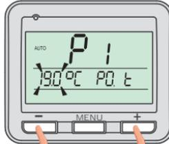
The desired temperature figure will start flashing. The temperature can be changed with the **+** or **-** buttons.
