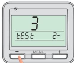
Send a signal to the second receiver by pushing the **-** button.
