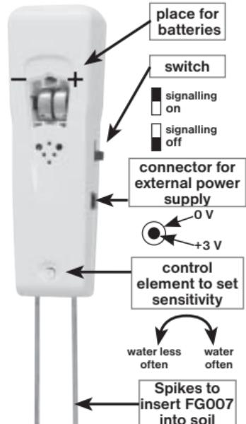
**Sensitivity setting:** Place the spikes of a FG007 into an optimally moist flowerpot. Use small screwdriver to turn the potentiometer into an utmost right position. Move the switch to an upper position and wait for the signal. Turn the potentiometer slowly to the left until the FG007 stops signalling. Setting is finished.
