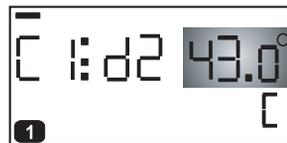
If the floor temperature achieves maximum permitted value, the thermostat will be switched off in case when temperature of the measured room did not achieve the required level. The thermostat will be switched on again when the external sensor temperature drops by 0.5°C.
