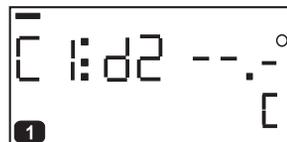
At Function 2 (page 5) it is possible to set another maximum temperature in range from 15 to 99.5°C. The temperature is measured by the external sensor. The advantage is that it is possible to measure the temperature in other room than in which the thermostat is placed (regulation of the temperature of water, floor, technological processes etc.).
