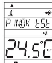
Signalizes correct connection of the module, but incorrect PIN code setting! It is necessary to disconnect the module, RESET central unit and set correct PIN code!
