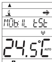
The module is not connected, incorrect connection of the module!
