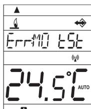
Signalizes correct connection of the module and PIN code setting.
