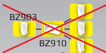
Improper assembly arrangement of bell and signal repeater!
