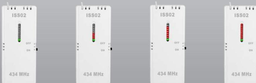
**Green LED lit.** No signal from transmitter, even from interference source.
