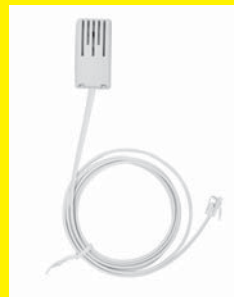
CT03-10k C order No. 0014 10kΩ, CYXY 2*0.5 mm, length 1.5 m, plastic case, for measurement to 70 °C
