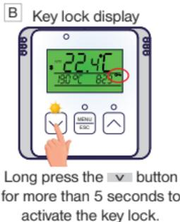
Long press the
