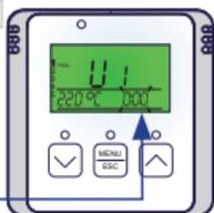
U1 (1st temperature change) appears on the display. Set the temperature with the / buttons and confirm with the MENU button.
