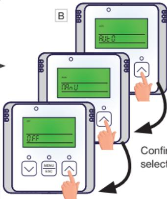
The **▲** / **▼** buttons can be used to select the desired **AUTO** or **MANU** or **OFF** mode.
