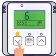
Press the button to send the signal to the second receiver.
