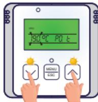
The required temperature will start flashing. The required temperature can be changed with the ▲ or ▼ buttons.
