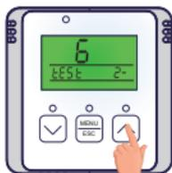
Press 1x button and „test 2-“ will appear on the display.
