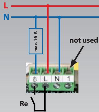
**Electronic room thermostats, controlled by microprocessor with external sensor.**
