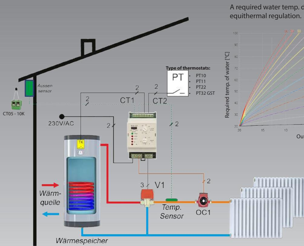
A required water temp. depending on outdoor temperature for equithermal regulation.
